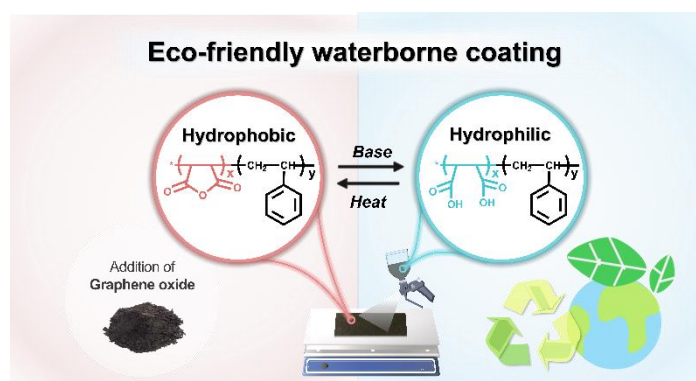
Figure 1. Schematic illustration of the ring-opening and ring-closing reactions of maleic anhydride (MA) units in the polarity-switchable MA-based copolymer
